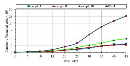
Fig. 7. Results of Acidithiobacillus thiooxidans bacteria counting for samples I, II, III, and the blank in the biofilm test stage.
