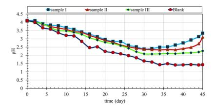
Fig. 4. Variation of the pH in the electrodeposited for samples I, II, III, and the blank in the pilot stage.
