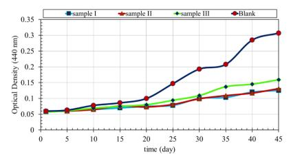
Fig. 6. Variations of optical density (OD) at 440 nm in the turbidity analysis during biofilm test stage.
