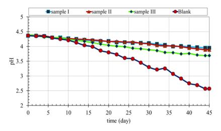
Fig. 5. Variation of the pH in the electrodeposited for samples I, II, III, and the blank in the biofilm test stage.
