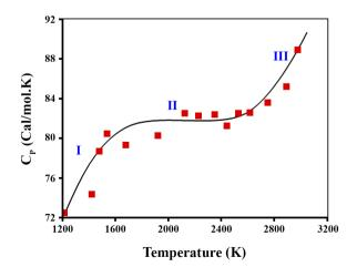
Fig. 1 Average heat capacity of zirconium dioxide versus temperature.
