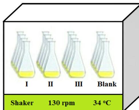
Fig. 3. The schematic of biofilm test stage (sample incubation).
