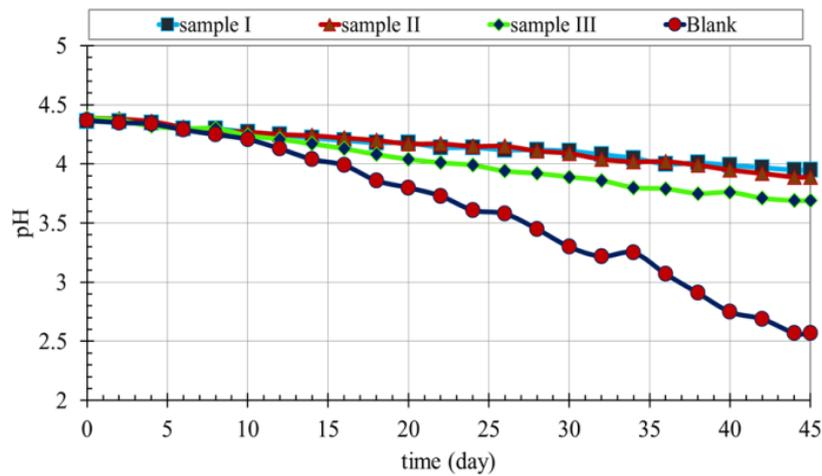
Fig. 5. Variation of the pH in the electrodeposited for samples I, II, III, and the blank in the biofilm test stage.
