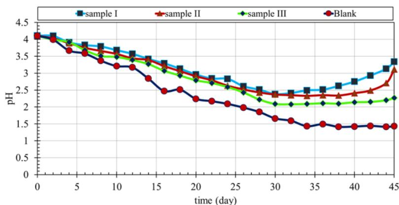
Fig. 4. Variation of the pH in the electrodeposited for samples I, II, III, and the blank in the pilot stage.
