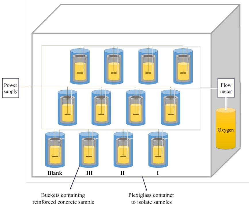
**Fig. 1.** The schema of the lab-scale pilot and reinforced concrete samples.
